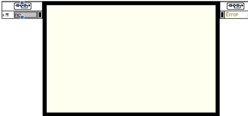
The Control & Simulation Loop has an Input Node (upper left corner) and an Output Node (upper right corner). Use the Input Node to configure simulation parameters programmatically. You also can configure these parameters interactively using the Configure Simulation Parameters dialog box. Access this dialog box by double-clicking the Input Node or by right-clicking the border and selecting Configure Simulation Parameters from the shortcut menu.
